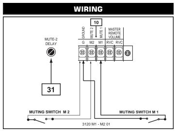
Fig. 17 - Direct Muting Terminals and Diagram
